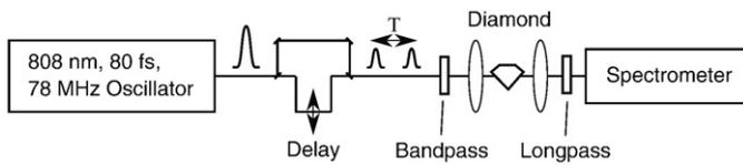
**Fig. 1.** Experimental setup. An oscillator pulse is split into two time delayed pulses and focused through the diamond sample. A bandpass filter removes background oscillator modes before the diamond and a longpass filter rejects the pump and transmits the Stokes before the spectrometer.
