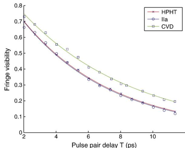
**Fig. 5.** A plot of spectral fringe visibility versus path delay set by the interferometer. These are typical runs obtained from the 3 diamonds.
